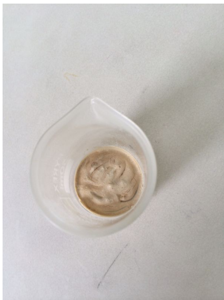
Illustration 5: Aspect du nylon chauffé
